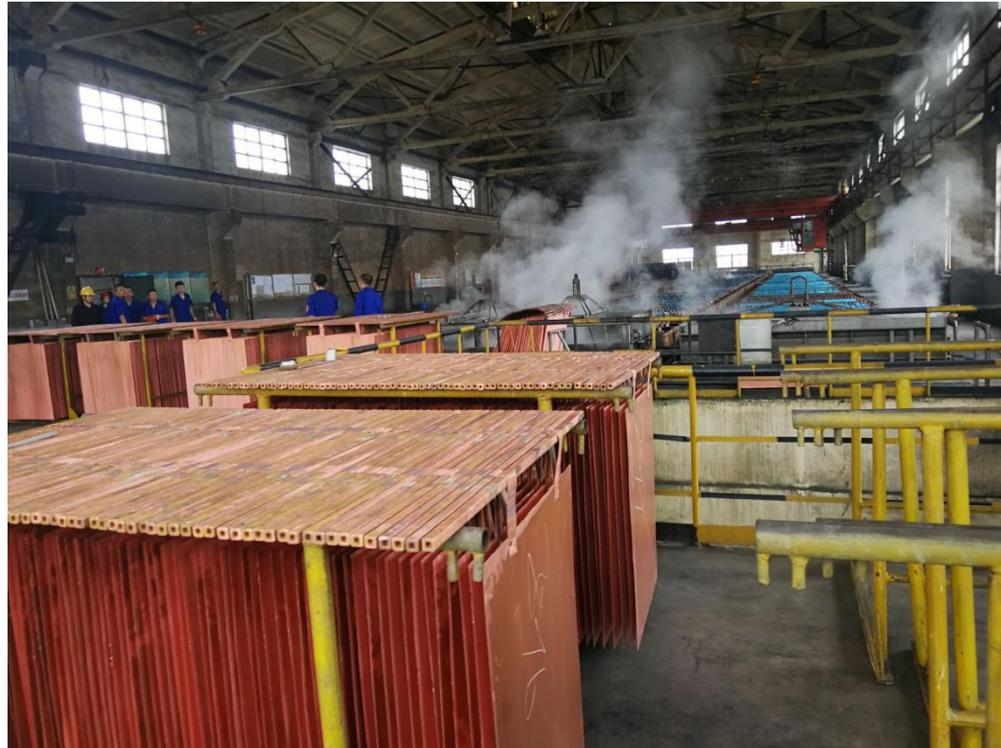
The copper electrolysis plant uses the electrolysis technology to purify and enrich copper. The main equipment in the electrolysis plant includes electrolyzers and corrosive materials, electrolytes and circulating pipes, pumps, ventilation facilities, and anode and cathode units.
